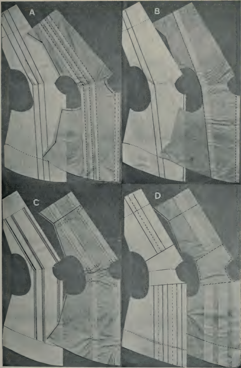
FIG. 69.—Method of designing waists from flat pattern; A , tucked or plaited waist; B waist with Gibson plait; C , box plaits and tucks D , box plaits with yoke.
